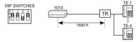
Figure 10—Extended Passive Bus (Linear)
